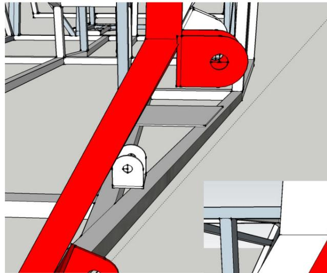
Showing the top bracket correctly aligned to suit the MX5 based wishbones on a standard Haynes designed chassis. As can be easily seen there is insufficient metal to make a good weld and the bracket, being that the geometry is 6mm narrower overall, needs rebating into the frame.
